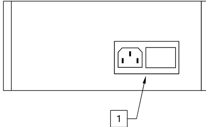
1. AC POWER INPUT. A three-pronged recessed male connector is provided on the back panel for AC power connection to the instrument. Also contained in this assembly is a slow blow fuse and a removable card that can be removed and repositioned to switch between 120V AC in and 240V AC in.
