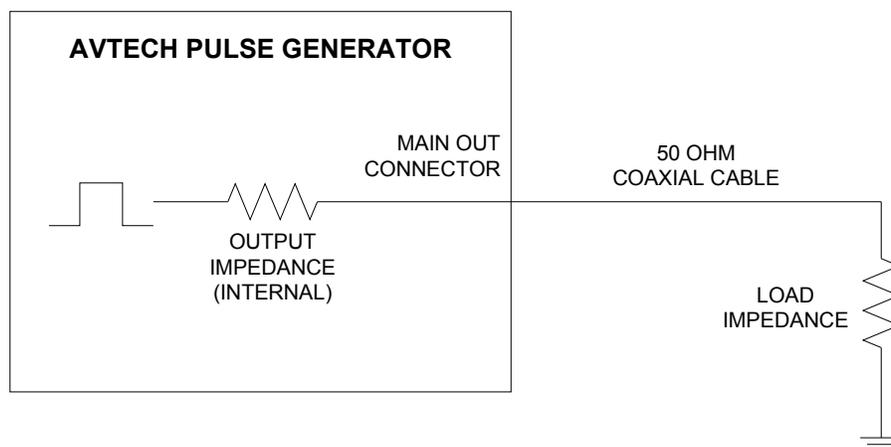
However, to obtain output amplitudes greater than  $\pm 5\text{V}$ , the  $\pm 10\text{V}$  ranges must be used, and the output impedance will be  $2\Omega$ . This is slightly less ideal, but good waveforms will still be obtained since the transmission line is still properly terminated on one end (the load end) with  $50\Omega$ .
