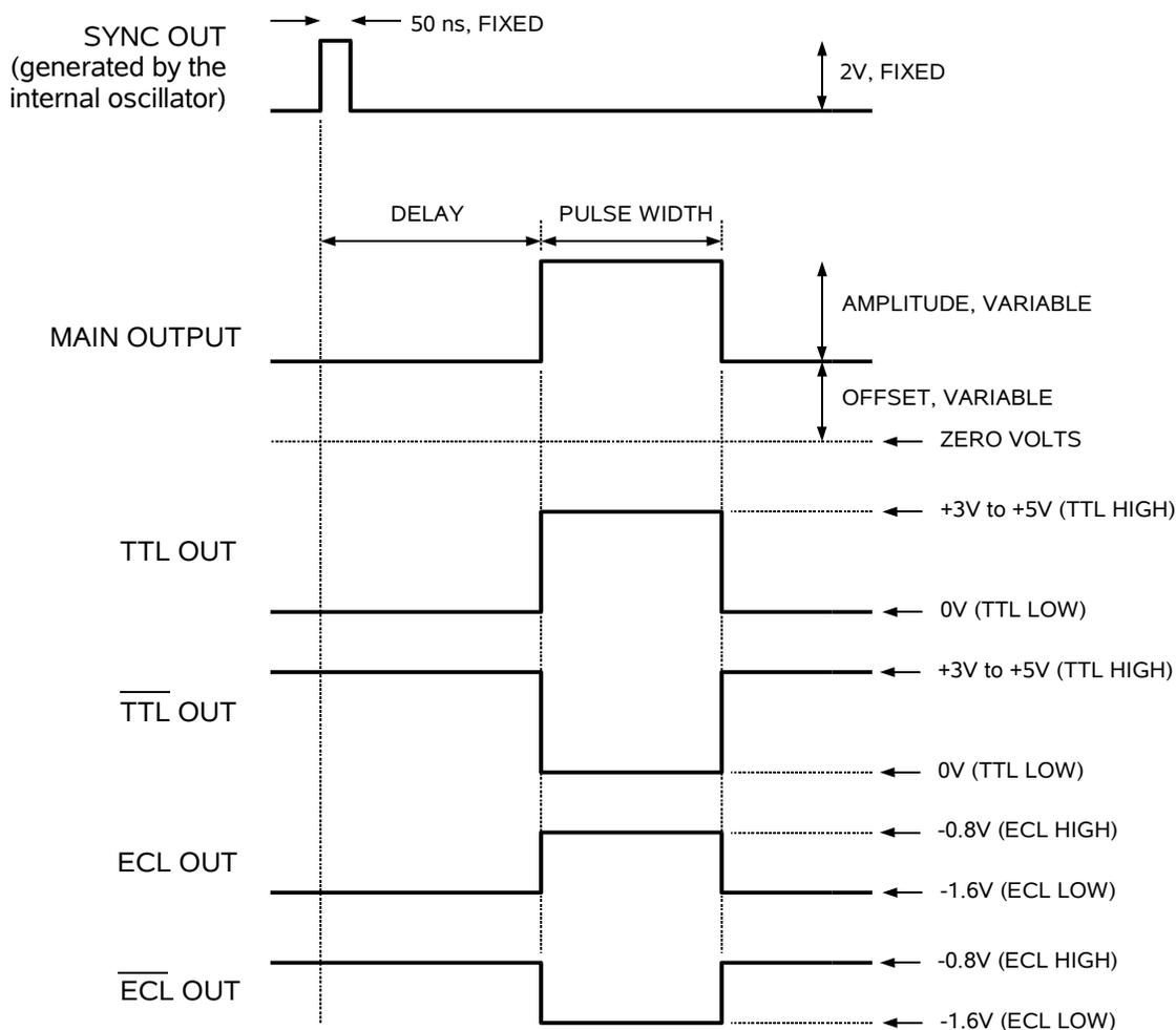
The next figure illustrates the relationship between the signals when an external TTL-level trigger is used (i.e., the REPETITION RATE switch is set to “EXT”):
